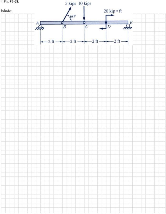
2-76 to 2-81 Replace the loading on the beams shown in Figs. P2-76 to Fig. P2-81 with an equivalent resultant force and specify their location along each beam measured from the left-hand end A.
