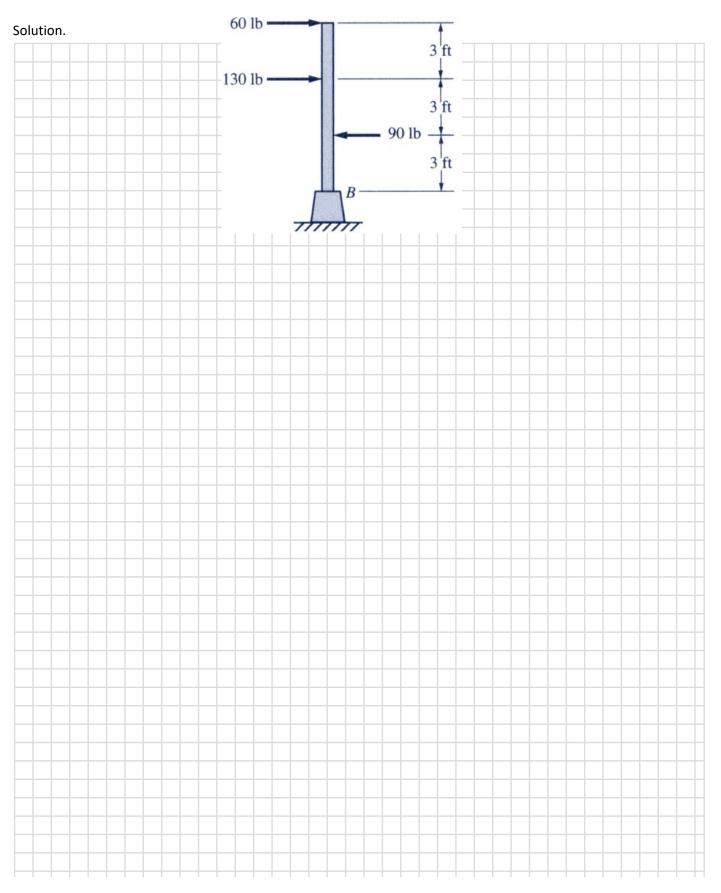
Determine the magnitude, direction, and location of the resultant of the two forces and a couple acting on the beam in Fig. P2-68.
