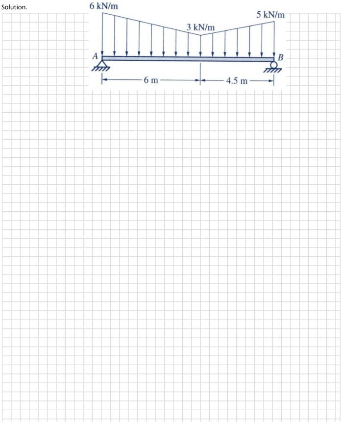
2-83 and 2-84 Replace the loading on the brackets in Fig. P2-83 and Fig. P2-84 with an equivalent resultant force and specify its location along AB mea-sured from a convenient point.
